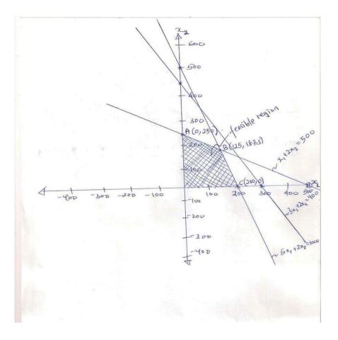
B is the point of intersection of lines  $x_1 + 2x_2 = 500$ ,  $5x_1 + 2x_2 = 1000$  on solving we get B = (125, 187.5)
